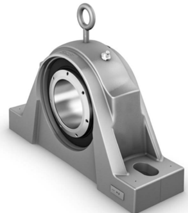
P2BA The cast-iron, two-bolt base pillow block unit with SAF dimensions. This makes for easy replacement when the features of a spherical roller unit are needed. See pages 320 and 321.
